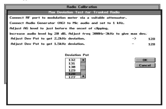
Set the audio generator to 1kHz and set the test unit 'Tx Audio' switch to 'Mic Audio'.
