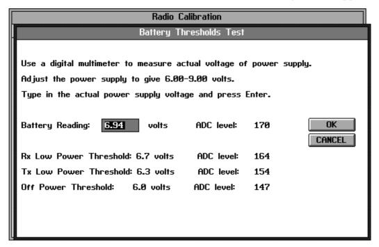
Adjust the power supply to give between 6 and 9V (normal battery voltage is 7.2V).
