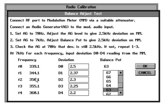
Connect the RF output of the radio to the modulation meter via the attenuator.
