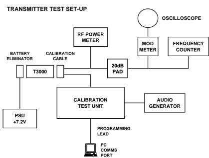
Figure 4.1 Test Equipment Set-Up
