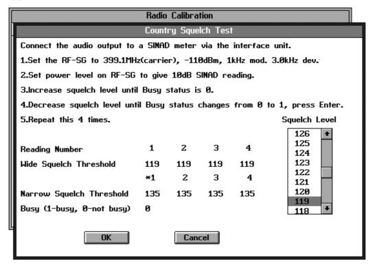
Connect the RF output of the radio to the RF signal generator via the attenuator. Connect the 'Sinad' audio output on the test unit to the sinad meter.
