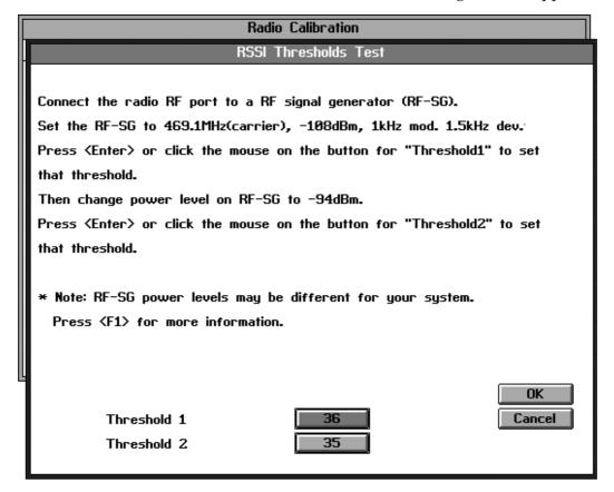
Connect the RF output of the radio to the RF signal generator via the attenuator. Connect the 'Sinad' audio output on the test unit to the sinad meter.
