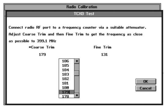
Connect the RF output of the radio to the frequency counter via the attenuator.
