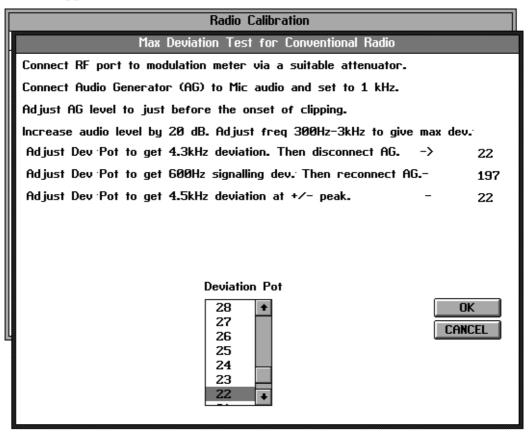
Set the audio generator to 1kHz and set the test unit 'Tx Audio' switch to 'Mic Audio'.
