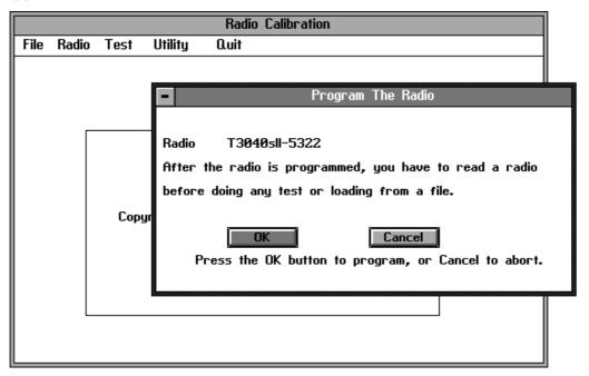
When the window opens, the **OK** button is highlighted. Press ENTER  $(\delta)$  to select **OK** button and the calibration data is entered into the radio's database.
