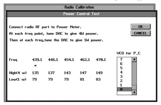
With the RF output of the radio connected to the power meter, the radio is set to transmit at each of the five points in the band.
