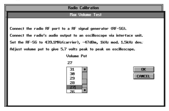
Connect the RF output of the radio to the RF signal generator via the attenuator and connect the 'Sinad' audio output on the test unit to the oscilloscope.
