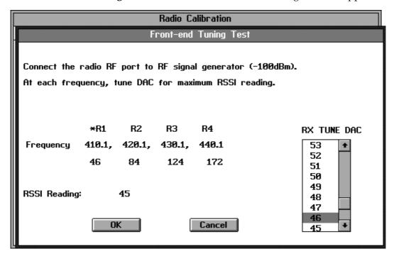
Connect the RF output of the radio to the RF signal generator via the attenuator. Connect the 'Sinad' audio output on the test unit to the sinad meter.
