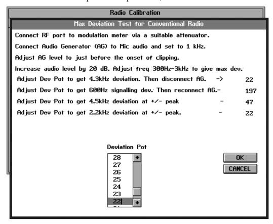
Readjust the **Deviation Pot** for  $\pm 2.2$ kHz deviation at the frequency of maximum deviation, and press ENTER ( $\downarrow$ ).
